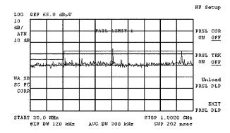
Figure 1a. Without preamplifier
